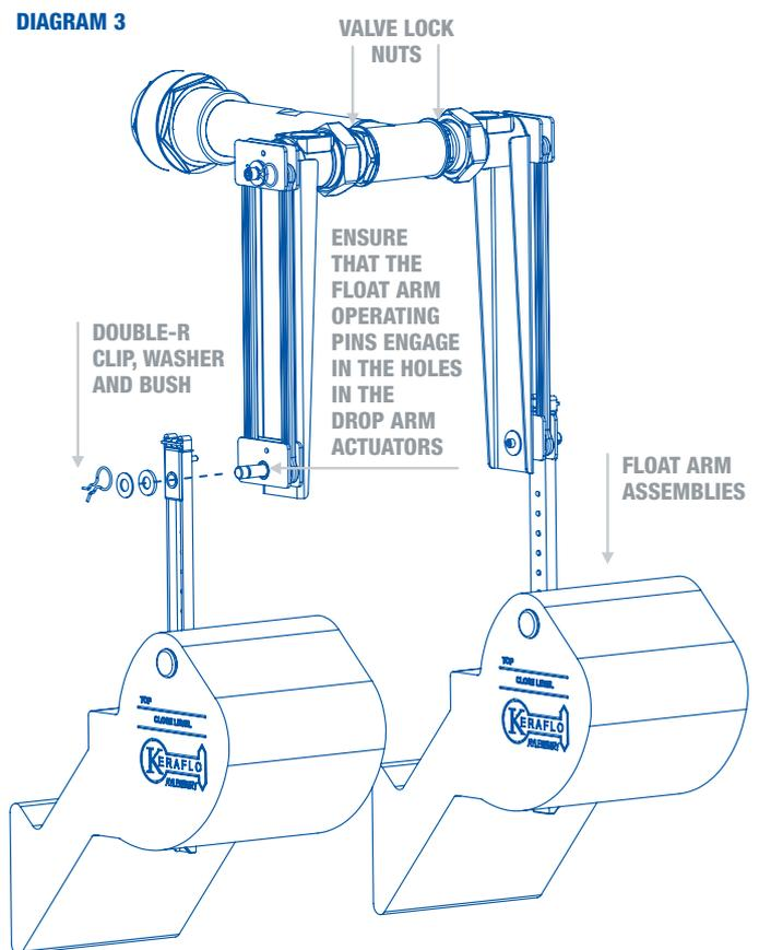
**10** If the valves are not level, each individual valve can be rotated at its screwed connection into the T-outlet. This joint is sealed by an “o”-ring so can be moved without fear of a leak.
