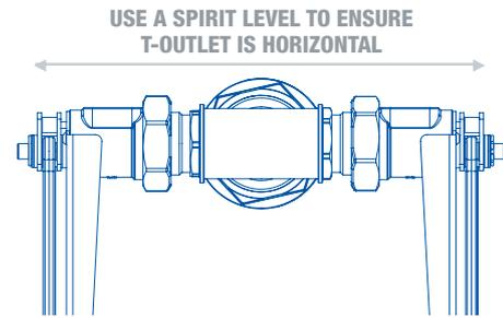
**8** Tighten the backnut sufficiently to hold the complete valve in position but note that it may be necessary to move the valve later after the float clearances have been measured.
