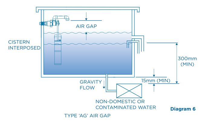
Water must flow by gravity only from the interposed cistern to the point of use. Furthermore a minimum head (pressure) must exist between the interposed cistern and the contaminated liquid as shown above. This arrangement should prevent contamination of the interposed cistern but convection and diffusion can cause chemicals to flow up towards the interposed cistern. However the mains supply is further protected by a Type 'AG' air gap inside the interposed cistern.
