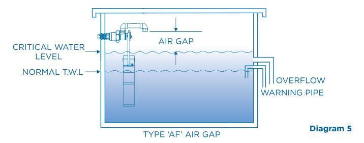
The critical level is the level the water will reach in a cistern should the float valve (or equivalent) fail and remain fully open e.g. punctured or removed float on BS1212 valves. All outlets except overflow/warning pipes must be closed and the supply pressure may be assumed to have a flow equivalent to a velocity of 3 m/s in the feed pipe.
