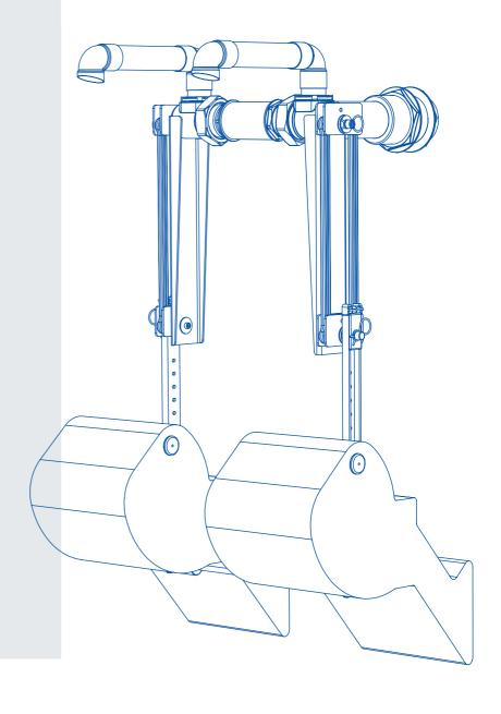
**KERAFLO** Aylesbury delayed action float valves contain a pair of maintenance free ceramic discs.
